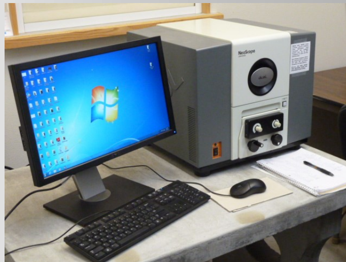
The Scanning Electron Microscope (SEM) used for imaging marine life at Friday Harbor.
